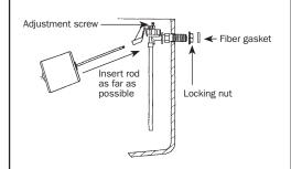
Manually screw the backnut until it is in contact with the ceramic. If necessary give an extra quarter turn (maximum). N.B.: Excessive tightening can damage the mechanism and would not be covered by the guarantee.
