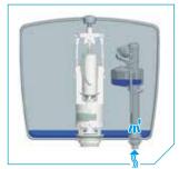
Once the flush is complete and the flush valve closes, the delaying case keeps draining water which then allows the inlet valve open and refill the cistern.
