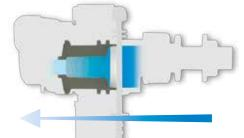
A case full of tiny marbles reduces the water pressure that comes through the inlet. This reduced flow makes the inlet ultra quiet.
