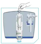
The cistern empties quicker than the water in the delaying case, keeping the inlet valve closed.
