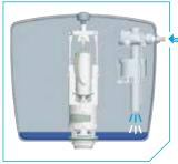
Once the flush is complete and the flush valve closes, the delaying case keeps draining water which then allows, the inlet valve open and refill the cistern.
